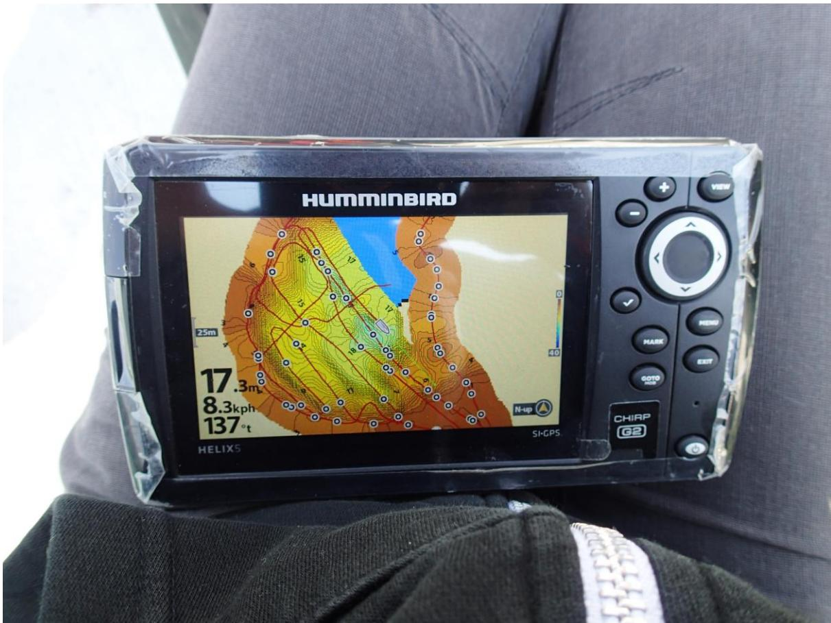
**Slika 6.:** Humminbird Helix 5 side-scan multi beam sonar
